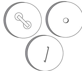
All O-Ring stoppers have handles. The 10" and 12" concrete stoppers have lifting holes, the 15" and above have handles. The plain clay stoppers have no handles. O-Ring stoppers can be wired or banded in O-Ring pipe.
